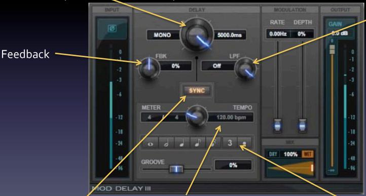
Low Pass Filter: A built-in filter that will cut out high frequencies. You can set the cutoff frequency.
